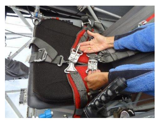
THE PILOT WILL BE WEARING THE PARACHUTE AND THERE'S NO NEED TO TAKE IT OFF BEFORE TAKING PILOT OUT OF COCKPIT IN AN EMERGENCY
