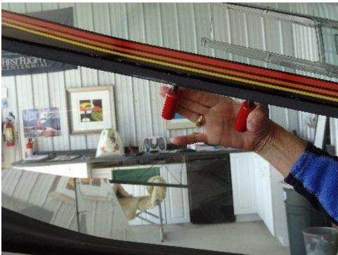
THE PILOT IS STRAPPED INTO THE COCKPIT WITH A 5 PLACE HARNESS THERE ARE TWO QUICK RELEASES THAT MOVE IN OPPOSITE DIRECTIONS PULL THE BOTTOM ONE LEFT AND THE TOP ONE RIGHT
